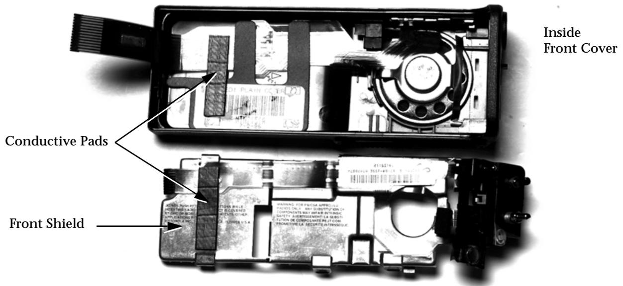
*Figure 1. Conductive Pad Placement*
